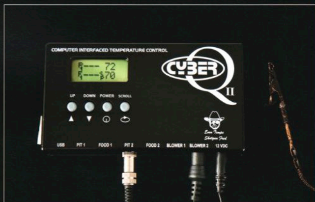
The CyberQ II is a controller system for barbecues that changes the temperature of smoke by regulating airflow to smoldering wood.
