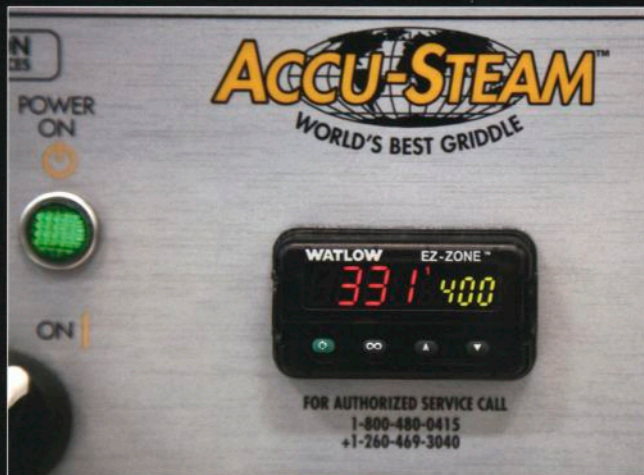
The PID controller on an Accu-Steam electric griddle replaces the simple control dial for greater accuracy.
