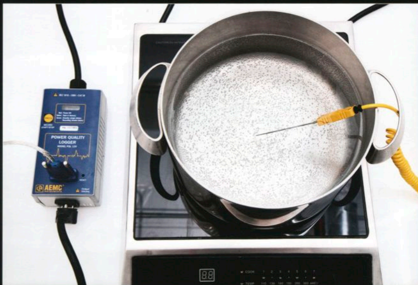
Our experimental setup for measuring thermal efficiency used a pot of water over the heating source under study, a thermal probe, and a data acquisition device connected to a computer.
