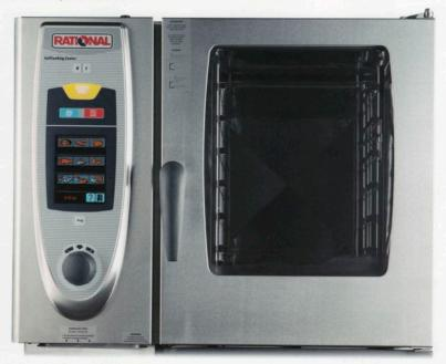
reservoir to generate humidity, combi ovens supply moisture directly, by injecting steam into the semisealed oven chamber. The combi oven's ability to use both steam and circulating hot and dry air, either alone or in combination, can reproduce, in a single appliance, many cooking techniques: steaming, proofing, incubating, dehydrating, baking, grilling, frying, and more. Cooks can program combi ovens to automate routine tasks, and the machines are self-cleaning.
