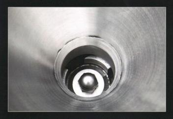
The hopper mouth typically incorporates a screw-feed mechanism that will force even a thick, viscous paste such as peanut butter into the mill.
