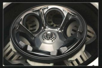
The standard rotor holds six bottles. Each bottle contains a different solution, but they all must be properly balanced.
