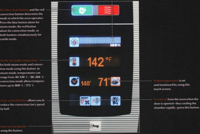
The blue steam button and the red .... convection button determine the mode in which the oven operates. Press the blue button alone for steam mode, the red button alone for convection mode, or both buttons simultaneously for combi mode.
