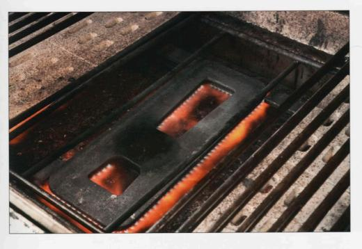
Clean-burning gas produces very little radiant heat directly. Gas grill manufacturers overcome this limitation by placing ceramic plates, lava rocks, or metal searing bars between the burner and the grill. The hot gases of combustion heat these objects until they emit a searing radiant heat that does the grilling. These hot surfaces also provide a place for drippings to fall and burn, thus contributing much of the flavor unique to grilling.
