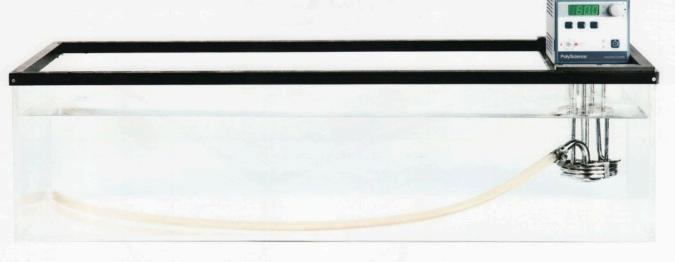
Circulating water baths designed to be plugged into a standard 120 V, 15 A North American outlet are generally limited to a volume of 30 I / 32 qt at most. Larger baths need more power than the electrical circuit can supply to keep the temperature even and stable.
