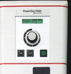
Splashing liquid can be a problem when you first engage the machine, so take the speed up slowly or in steps. A high-end rotor-stator homogenizer enables cooks to preprogram processing runs to avoid this problem.
