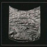
Heat-shrink bags compress food more tightly than a vacuum alone can. Molecules aligned in the bag are stretched when cool but shrink when heated, shortening the bag to about a quarter of its initial length.
