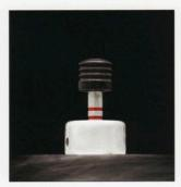
Spring-loaded valves are common on pressure cookers and generally unsuitable for canning because they can prevent proper venting and become inaccurate over time as the spring fatigues.
