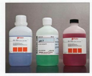
You can buy solutions formulated to exactly to pH values of exactly four, seven, and 10 (above and below) to use in calibrating you pH meter. Refer to the manufacturer's instructions to calibrate your meter, but most devices have a special calibration mode.
