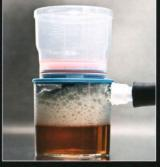
extremely fine membrane filter (220 nanometers or finer) and is disposable. It works in the same way as a Büchner funnel setup. You connect the apparatus to a vacuum pump with a rubber hose. The
