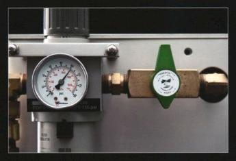
Compressed air provides the energy that drives most high-pressure homogenizers. The air comes from a machine-shop air compressor—the kind commonly used for spray-painting. Some homogenizers are electrically driven instead.
