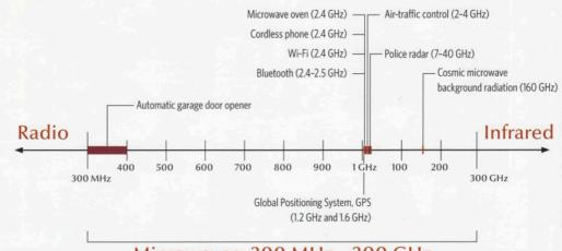
Microwaves are a form of electromagnetic radiation with frequencies between 300 megahertz (MHz) and 300 gigahertz (GHz). Microwave ovens, cordless phones, and wireless Internet connections all operate at frequencies near 2.4 GHz, which cannot be used for long-distance signals, because water molecules in the atmosphere interfere with their transmission-the same phenomenon that makes these wavelengths perfect for cooking.
