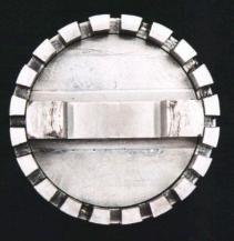
The generator comprises a rapidly spinning blade, called a rotor (center piece above), and a notched stationary piece called a stator. Although the rotor is not sharpened, its design and precise dimensions allow it to strike, with great force, food particles in a liquid, say, or oil droplets in an emulsion. As it pushes the food through notches in the stator, high shear forces are imposed on food particles in the small gap between the rotor and stator.
