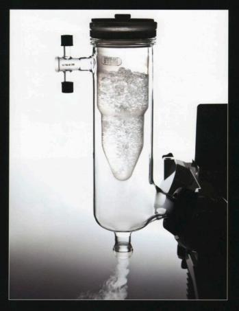
A cold trap can use dry ice, liquid nitrogen, or ice mixed with salt to cool the most volatile vapors more effectively than a condensing column can.
