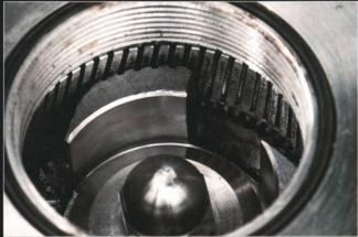
The rotor-stator assembly is the business end of the colloid mill. This part of the tool resembles a similar device on a rotor-stator homogenizer, except that the mill forces all the material through the rotor-stator without requiring the cook to stir it. The device applies a powerful combination of shearing, grinding, and high-speed mixing forces to reduce the size of the particles in the fluid.
