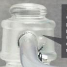
The side port connects to a vacuum pump, which evacuates air from the container. On the glass container shown here, twisting the side port aligns or separates holes to evacuate or seal the chamber. On plastic vessels, a separate stopcock can be rotated to accomplish the same function.
