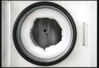
After the water in the food sublimates, it refreezes as ice on the coldest thing around, which is the condenser (also called a cold trap)—not the food. For freeze dryers of moderate size, the capacity of the condenser ranges from 5-25 kg / 11-55 lb and limits how much food the dryer can process at once.
