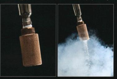
Liquid nitrogen can be dispensed by pouring or, for large Dewars, by using a special dispensing system.
