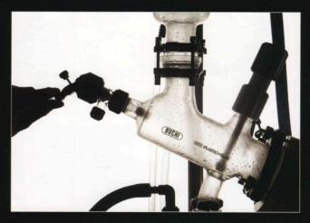
The vacuum pump system includes several vacuum joints and control valves from which you can bleed off vacuum when needed. To keep the system free of leaks that can cause the process to fail, you must carefully seal all the joints.
