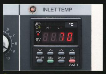
2 Set the temperature of the liquid spray. Use the dial at the top of the machine to set the spray or inlet-control temperature. We have found 70 °C/160 °F to be a good starting point for kitchen-scale machines.
