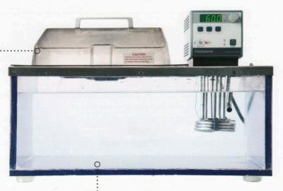
A portable immersion circulator with digital controls can be used in baths of various sizes and designs.
