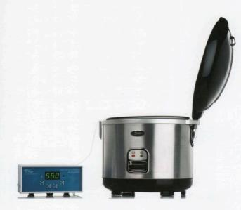
PID controller added to an existing appliance Examples: PID-controlled crock pot or rice cooker,
