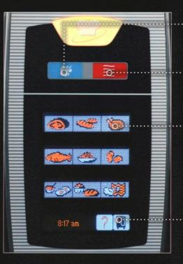
The steam-mode button, when pressed alone, injects steam at oven temperatures from 30-130 °C / 86-266 °F.
