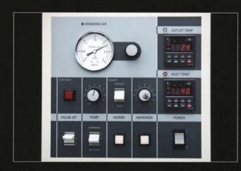
The controls typically allow you to set the rate at which the liquid is sprayed into the chamber (via the pressure of the "atomizing air" in the spray nozzle). You can also adjust the temperatures of the inlet air, the outlet air, and the liquid itself. A fair amount of trial and error is required to find the optimal temperatures for different liquids.
