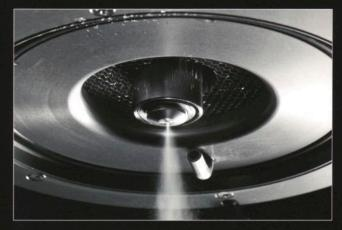
The injection nozzle atomizes the fluid into a mist of droplets that range in diameter from 180-250 microns / 0.007-0.01 in.
