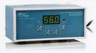
This add-on PID controller is made to be used with "dumb" devices like crock pots and rice cookers; it gives them the "smarts" to control temperature accurately. Immersion circulators and water baths have similar control logic circuits built into them.
