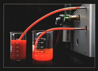
The homogenizer takes fluid from an input flask (at right, above), processes it, and sends the result to an output flask (at left). The machine simply sucks in thin liquids, but thick liquids and purees, ranging in consistency from mayonnaise to ketchup, will flow into the narrow inlet only if fed from a pressurized hopper.
