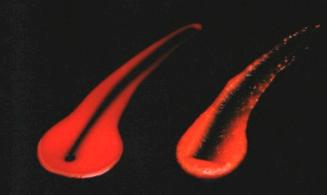
A pass through the machine significantly reduces the size of the particle in the fluid. You can clearly see the marked difference in texture between the grainy material before (right) and the silky smooth liquid after (left) a single pass through the high-pressure homogenizer. Successive passes increase the uniformity of the particle sizes.
