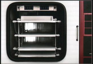
The shelves are temperature-controlled. Typically, you set them initially to about 20 °C / 36 °F above the critical freezing temperature of the food; they then supply the heat that drives the sublimation process. You later increase the temperature as much as is practical to finish drying the food.
