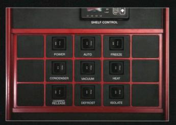
Control units vary widely from one model of freeze dryer to another. But all devices allow you to set the vacuum pressure, the shelf temperature, and the condenser temperature.
