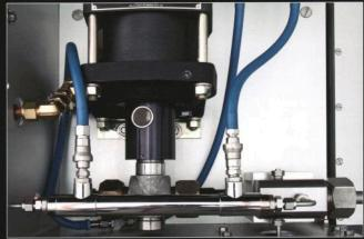
The pressure pump is one of the crucial elements of a high-pressure homogenizer. The design of the pump system and its valves allow the liquid to be moved around, pressurized, and then depressurized after processing it in the impinger.
