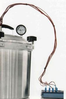
We built a pressure canner with multiple thermocouple probes to test temperatures in all phases of the canning process.
