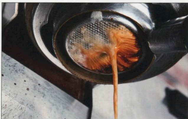
Uneven flow comes from uneven dosing, grooming, and tamping. It creates a bad shot.
