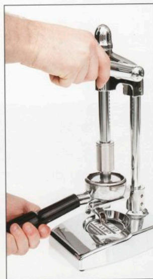
The auto-tamp includes a built-in gauge that clicks when the appropriate force has been applied. That feature makes it easier to apply the same pressure each time, which otherwise takes some practice. A frame also ensures that the tamping pressure is always directly vertical and never skewed.
