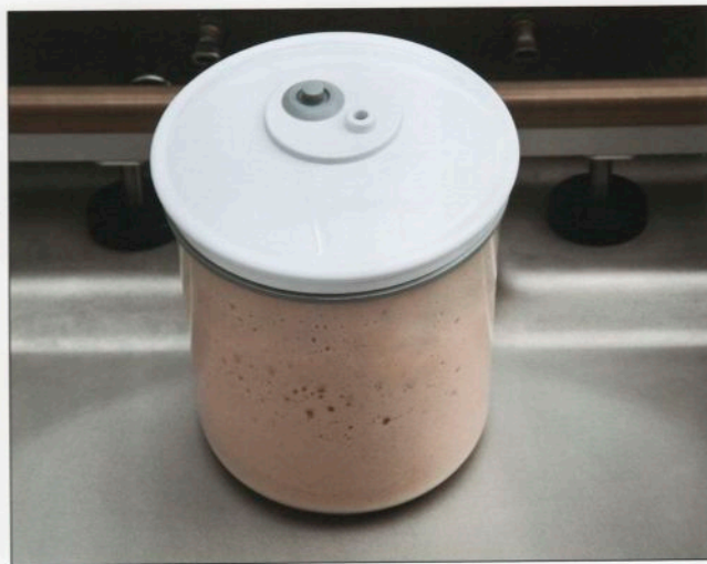
Sucking air out of the container with a vacuum pump expands the foam greatly, and it can now set in this expanded state.
