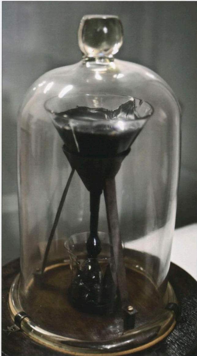
Since the pitch drop experiment was first put on display at the University of Queensland in 1927, just eight drops have fallen out of the funnel full of pitch.
